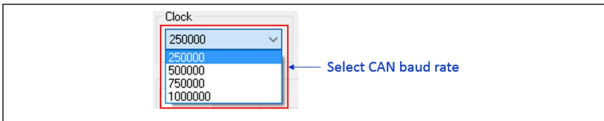
Figure 4-16 Change CAN Baud Rate
